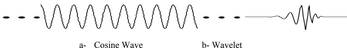
Figure(2):Continuous sinusoid and continuous wavelet
